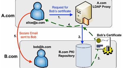
Carillon's Simple•CDS<sup>™</sup>LDAP Proxy is built on top of version 2.3.43 of the OpenLDAP open-source LDAP server and a heavily modified version of the open-source "getcert" back-end module originally written by The Boeing Company.
